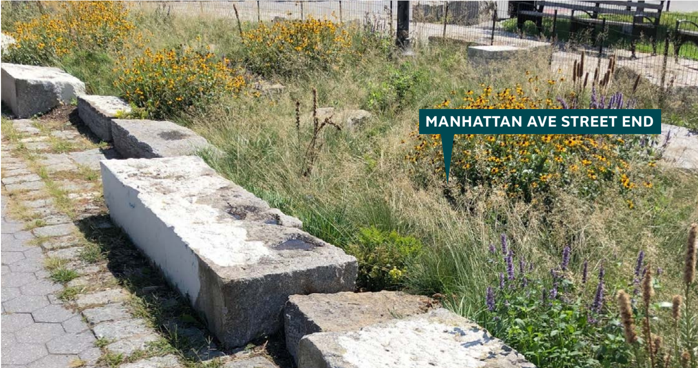
PLANT BEDS WITH BOULDERS TO PROVIDE STORM SURGE BUFFER AND SEATING
