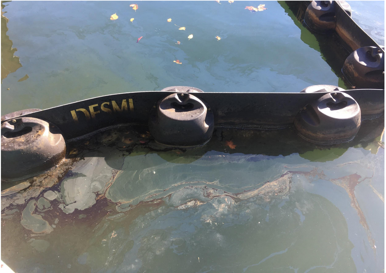
Petroleum on both sides of containment boom. November 2016.
